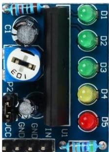
A KA2284 Module this is a small signal meter for audio devices and is the module we are going to hack to get our signal for the jaw to respond to.
