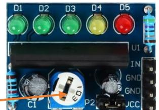
The sensitivity of the movement is controlled by the Potentiometer located on the KA2284 board. You will have to fiddle with it based on the loudness of your MP3s.
